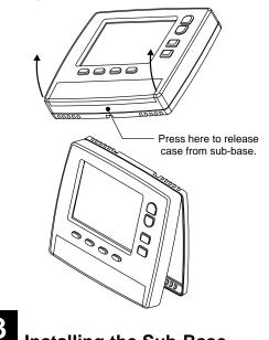
The thermostat can be installed on any interior wall approximately 5 feet above the floor. To insure accurate reading of the space temperature, the thermostat should not be
